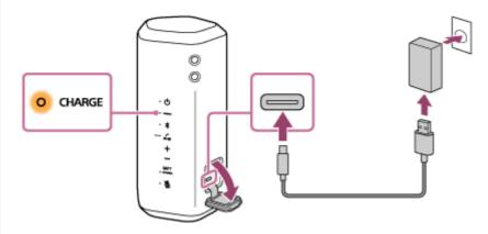
The CHARGE indicator lights up in orange<sup>\*1</sup> while charging is in progress.
